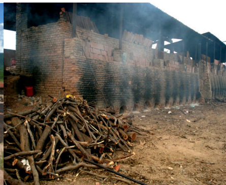
“Caipira kiln” for roof-tile production.
