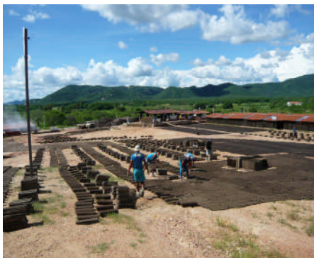
Drying of roof tiles in a small roof-tile production company in Carnaúba dos Dantas, RN.
